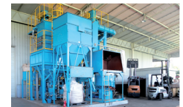
Mixer for recycling casting sand
