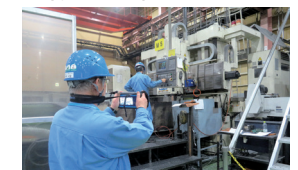
Air leak examination
